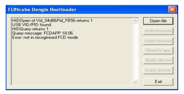
Line 4 indicates the firmware version installed.
