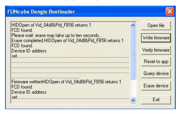
If you scroll to the bottom of the text box it should end with the words "Firmware verified".
