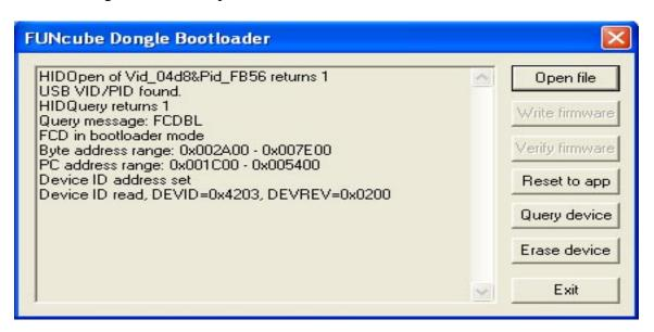
Click on "Open file", the following window will open allowing you to navigate to the location in which you saved the firmware binary file.
