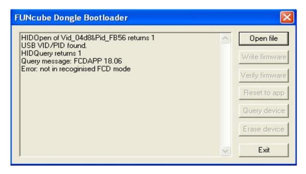
Notice the fourth line down in the text box: "Query message: FCDAPP 18.06" This identifies the firmware version loaded, in this case 18.06 = v18f. For more information see "Using the Bootloader to Identify Firmware Version" below.
